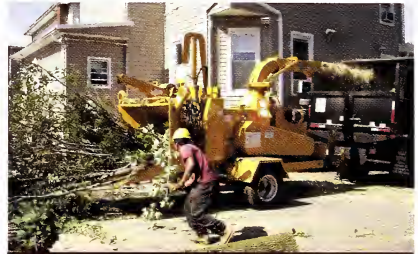
Figure 6. Regulated materials chipped to less than 1 inch in two dimensions can move out of the regulated area.
